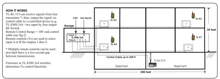
Figure 3 Example Application RF Remote Control for RF Signal Switcher in small building
