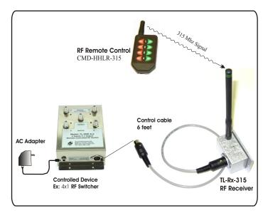
Figure 1 RF Remote Control for RF Signal Switcher
